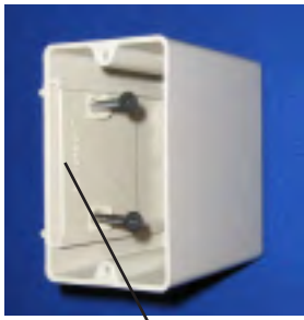
Slider plate in full forward position sets box for 1/2" drywall.
