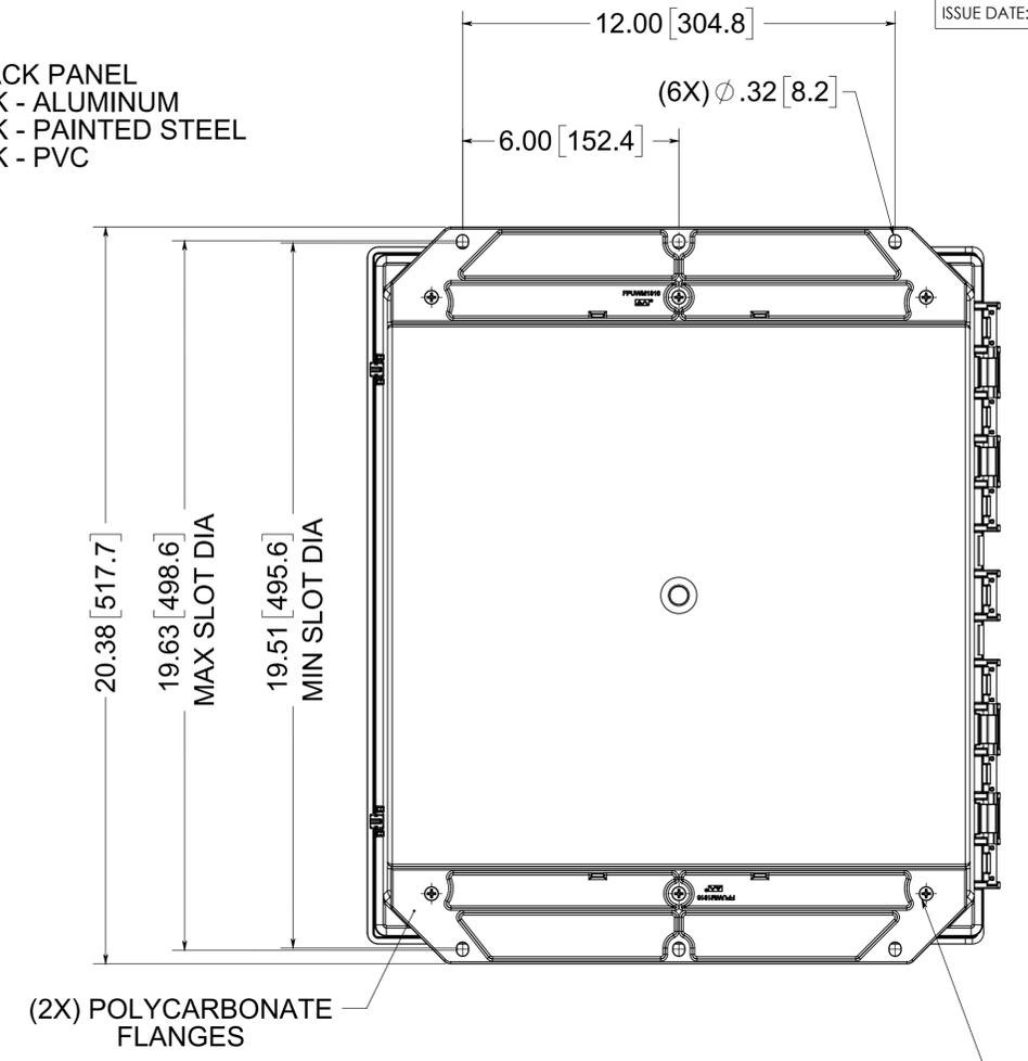
(4X) SNAP-IN POLYCARBONATE HINGE KNUCKLE
