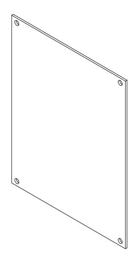
Aluminum 3002-H14 With Protective Peel-Off Film
