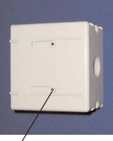
Slider plate in full forward position sets box for 1/2" drywall.
