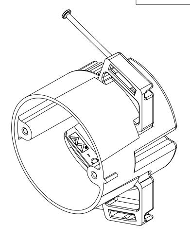
1.) BOX MATERIAL: FIBERGLASS REINFORCED POLYESTER, NAIL MATERIAL: PLATED CARBON STEEL, WIRE CLAMP MATERIAL: GALVANIZED STEEL, WIRE CLAMP SCREW MATERIAL: ZINC PLATED STEEL
