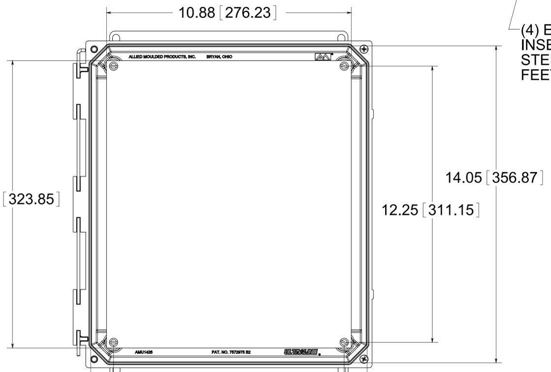
(4) EACH #10-32 BRASS INSERTS, AND STAINLESS STEEL FLANGE AND FEET SCREWS
