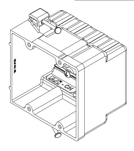
1.) BOX MATERIAL: FIBERGLASS REINFORCED POLYESTER, NAIL MATERIAL: PLATED CARBON STEEL, WIRE CLAMP MATERIAL: GALVANIZED STEEL, WIRE CLAMP SCREW MATERIAL: ZINC PLATED STEEL
