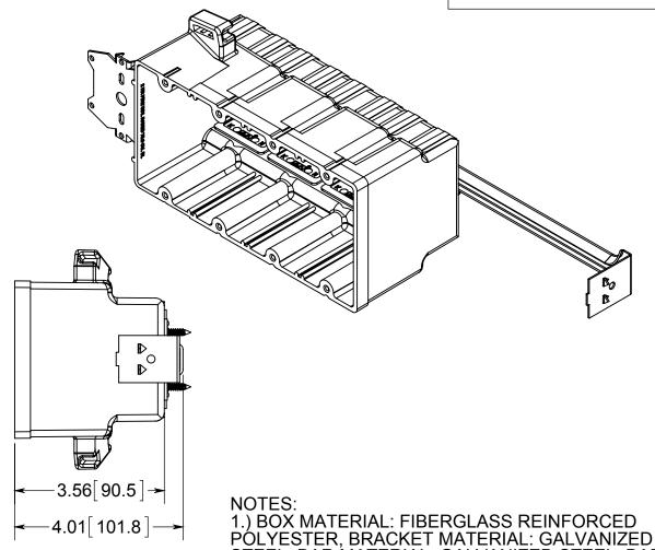
1.) BOX MATERIAL: FIBERGLASS REINFORCED POLYESTER, BRACKET MATERIAL: GALVANIZED STEEL, BAR MATERIAL: GALVANIZED STEEL, BAR MOUNTING BRACKET MATERIAL: GALVANIZED STEEL, BAR MOUNTING BRACKET SCREW MATERIAL: ZINC PLATED STEEL, SPEED KLAMP MATERIAL: PVC
