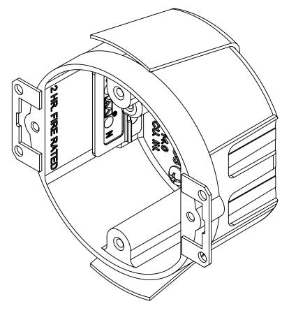
1.) BOX MATERIAL: FIBERGLASS REINFORCED POLYESTER, EAR MATERIAL: GALVANIZED STEEL, SNAP BRACKET MATERIAL: GALVANIZED STEEL, SNAP BRACKET SCREW MATERIAL: ZINC PLATED STEEL, SPEED KLAMP MATERIAL: PVC 2.) UL LISTED WITH 2 HOUR FIRE RATING FOR WALL AND CEILING 3.) 2 SPEED KLAMPS FACTORY INSTALLED
