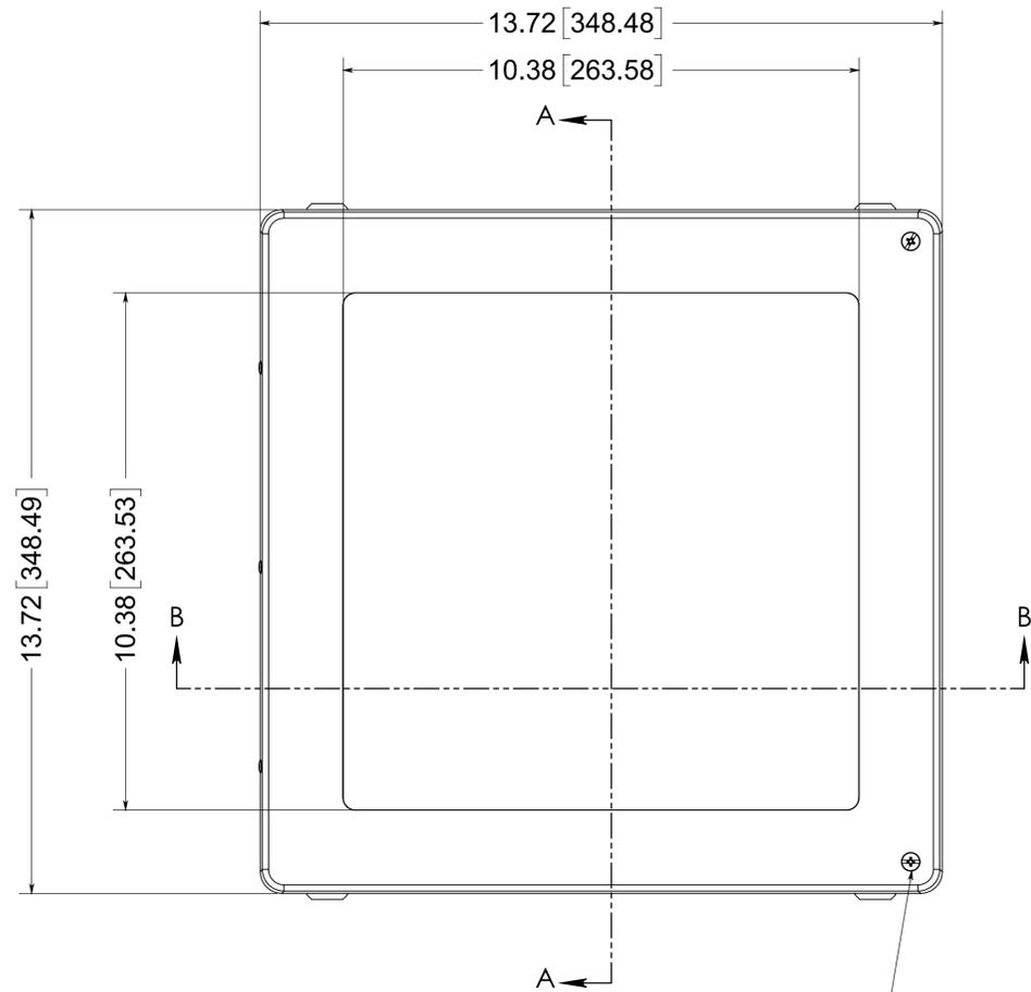
(2) EACH #10-32 BRASS INSERTS AND 316 STAINLESS STEEL CAPTIVE COVER SCREWS WITH RETAINING O-RING
