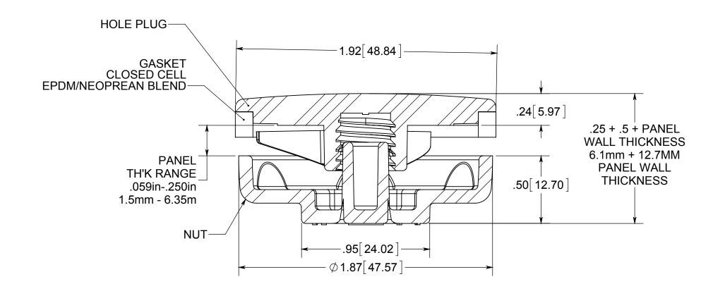
PLUGGED HOLE DIA RANGE: 1.375in-1.625in 34.93mm-41.28mm
