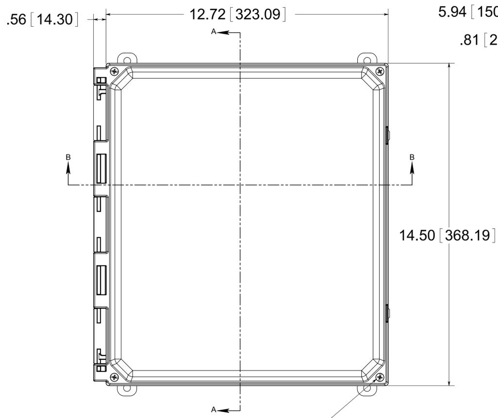
(4) EACH #10-32 BRASS INSERTS AND STAINLESS STEEL CAPTIVE COVER SCREWS WITH RETAINING O-RING
