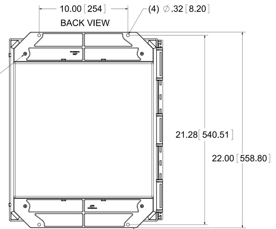
(4) EACH #10-32 BRASS INSERTS, AND STAINLESS STEEL FLANGE AND FEET SCREWS
