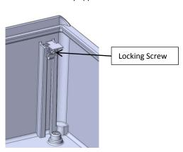
Step 3. Assemble the Swing Out Panel assembly onto the Hinge Side Brackets. Pull the spring loaded hinge device and align the hinge rod with the hole on the Hinge Side Bracket. Release the spring loaded hinge device to engage the hinge rod in the bracket. Repeat for the opposite side of the Swing Out panel.
