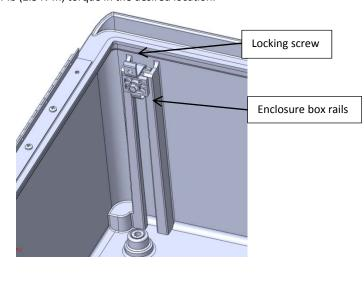
Step 2. Repeat Step #1 using the Latch Side Brackets. Note that the second Bracket set should be installed directly opposite the first Bracket set.
