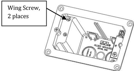
7. Alternate installation method: screw the box down directly to the floor using the four #6 wood screws through the countersunk holes in the flange of the plastic box.
