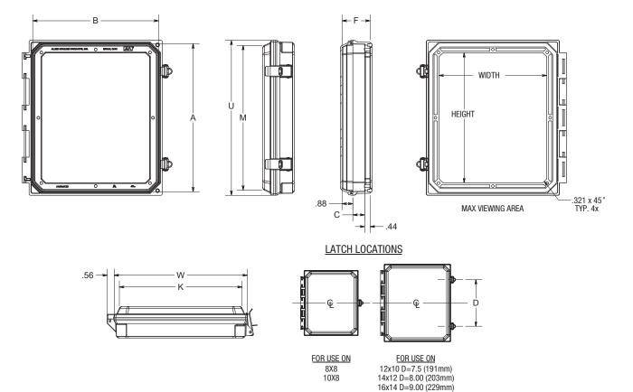
Note: For use on flat smooth surfaces of NEMA Types 1, 3, 3R, 4, 4X, 12 or 13 enclosures
